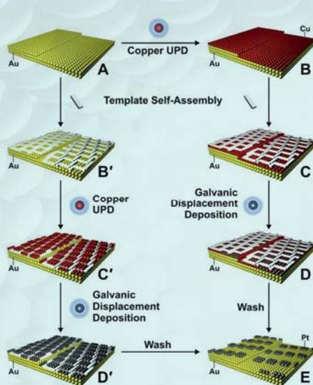
SLRR AND SUPRAMOLECULAR TEMPLATE SELF-ASSEMBLY STEPS TO PRODUCE ORDERED MONOLAYER PT CATALYST. PATH 1: A-B'-C'-D'-E, PATH 2: A-B-C-D-E
