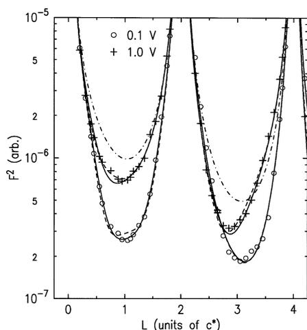
Fig. 5. Specular reflectivity (structure factor squared) measured for Ru(0001) at 0.1 V (circles) and 1.0 V (plus sign) in 1 M  $\text{H}_2\text{SO}_4$  with the dot-dash line showing the calculated curve for an ideally terminated Ru(0001). The dashed and solid lines are the fits discussed in the text.
