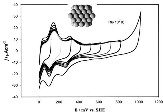
Fig. 2. Voltammetric curves of Ru(10–10) in 0.1 M  $H_2SO_4$  solution. Sweep rate  $10 \text{ mV s}^{-1}$ . Inset: a model of one out of two terminations of a Ru(10–10) surface.
