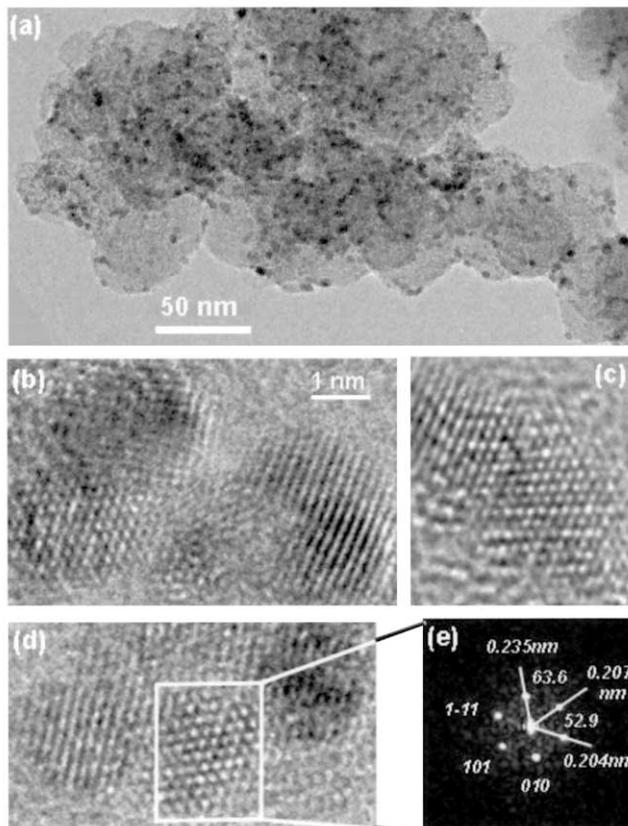
Fig. 9. Electron micrographs of Ru nanoparticles. (a) Low magnification morphology of the particles (black dots) on carbon spheres. (b–d) High-resolution images of the particles which have an average diameter of about 2.5 nm. (e) Diffractogram obtained from the high-resolution image shown in (d) (boxed area). Diffraction analysis reveals that the angles and lattice constants are consistent with the hcp Ru single crystal structure.
