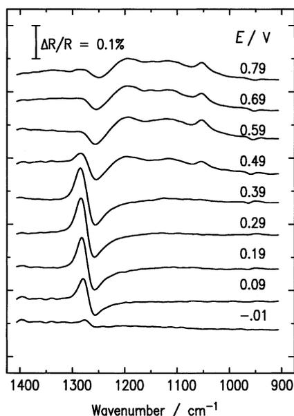
Fig. 3. In situ infrared spectra obtained from the Ru(0001) electrode in 0.05 M  $\text{H}_2\text{SO}_4$ . The reference spectrum is obtained at  $-0.03$  V vs. SHE, and sample spectra are taken every 0.1 V, from  $-0.01$  to 0.79 V. Scans (4096) were coadded in 16 cycles, 256 scans each; the resolution was  $8\text{ cm}^{-1}$ . Spectra are offset for clarity.
