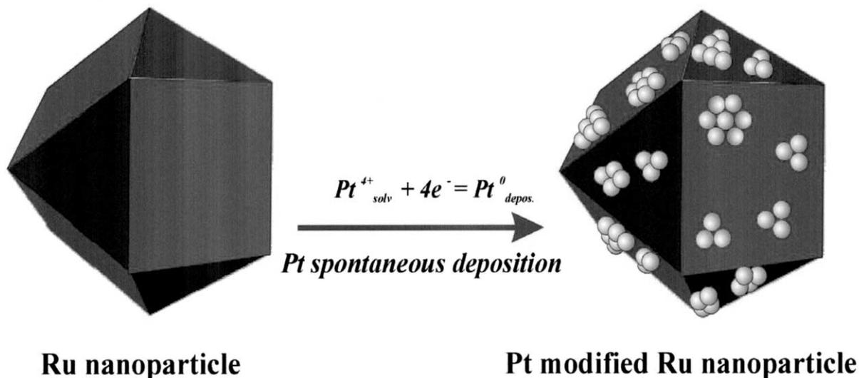
Fig. 8. Model of a cubo-octahedral Ru nanoparticle covered by 1/4 of a Pt monolayer.
