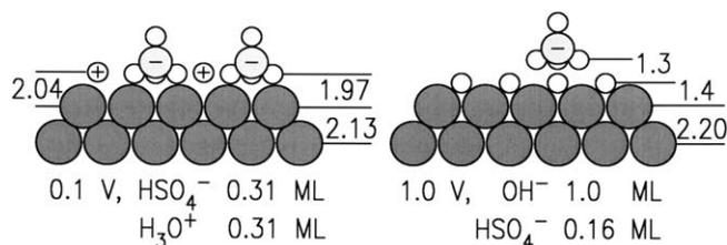
Fig. 6. Proposed schematics of structural models where the O, S, and Ru atoms are represented by the open, heavily shaded, and lightly shaded circles, respectively. The layer spacings are given in angstrom and coverages are given in monolayer (ML).
