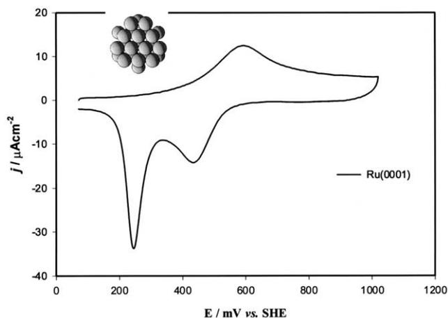
Fig. 1. Voltammetric curves of Ru(0001) in 0.1 M  $H_2SO_4$  solution. Sweep rate  $10 \text{ mV s}^{-1}$ . Inset: a model of a Ru(0001) surface.
