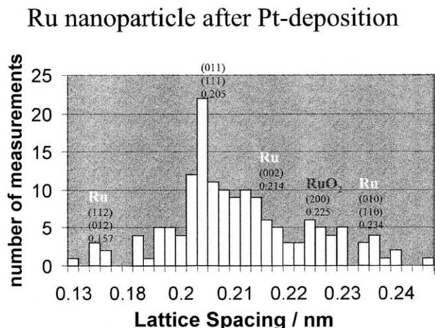
Fig. 10. Lattice spacing distribution of the nanoparticles measured from the high-resolution images ( $\sim 170$  measurements) showing that the particles are mainly metallic Ru with a small amount of  $\text{RuO}_2$ .
