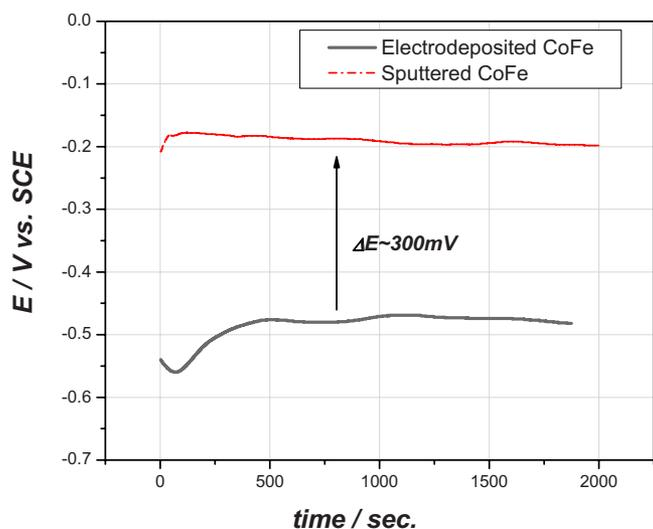
**Figure 1.** (Color online) The corrosion potential transients for sputtered (dashed) and electrodeposited 2.4 T CoFe alloy (solid line). Test solution: 0.5 M NaCl. Data adopted from Ref. 23.
