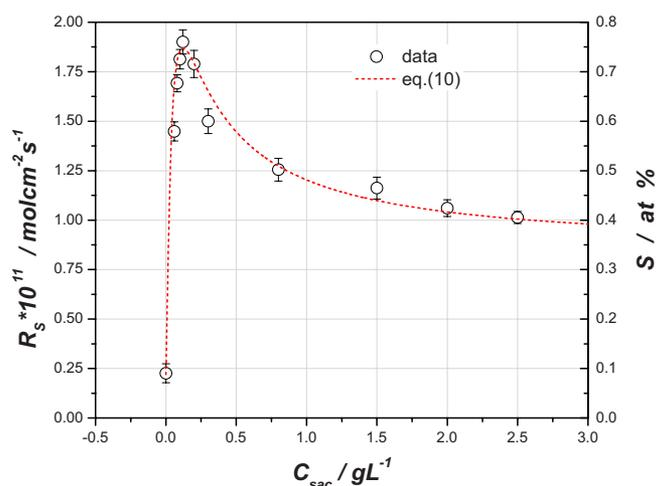
**Figure 2.** (Color online) The WDS measurements showing atomic percent of S as a function of saccharin concentration in the bath, (right ordinate), and corresponding sulfur incorporation rate (left ordinate) [Eq. 1].
