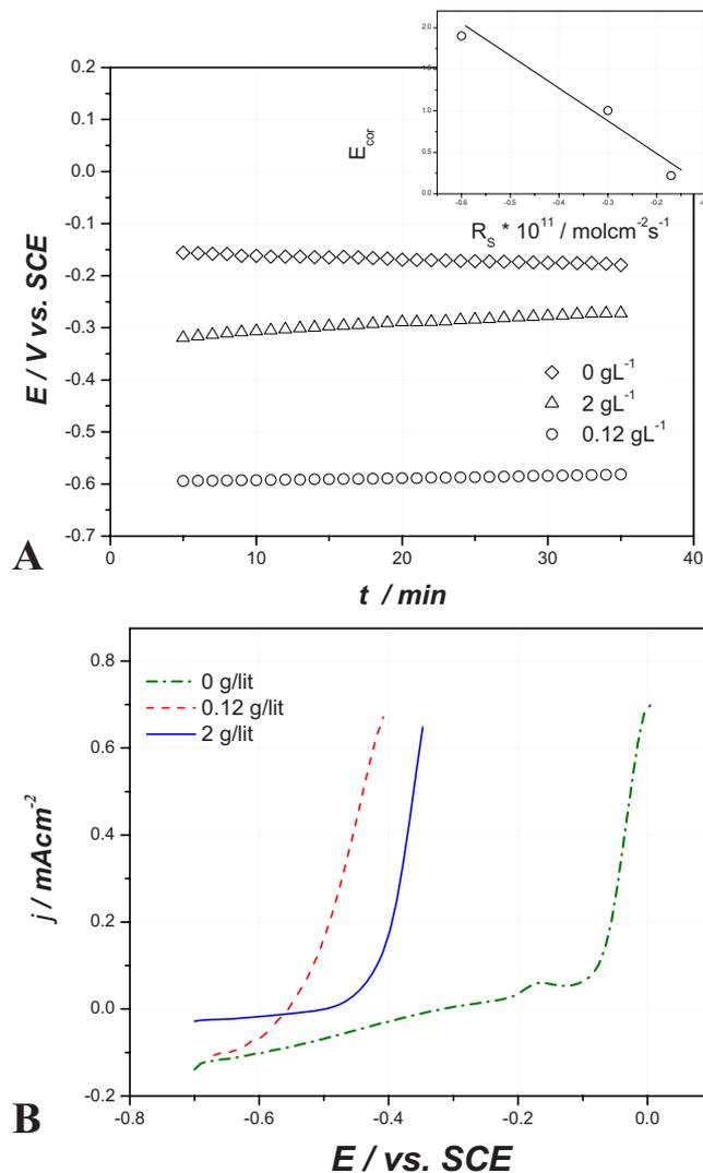
Figure 6. (Color online) (A) Corrosion potential transients for 2.4 T CoFe films electrodeposited from solutions containing 0, 0.12, and 2 g L<sup>-1</sup> of saccharin. The inset shows corrosion potential as a function of total sulfur incorporation rate. (B) Linear sweep voltammetry results for 2.4 T CoFe films electrodeposited from solutions containing 0, 0.12, and 2 g L<sup>-1</sup> of saccharin. The test solution in both cases is 0.05 M NaCl.
