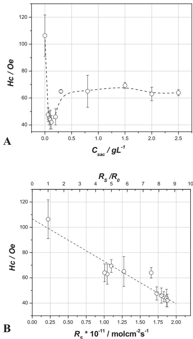
**Figure 4.** (A) Coercivity of 2.4 T CoFe alloys as a function of saccharin concentration in the plating solution. (B) Coercivity of 2.4 T CoFe alloys as a function of sulfur incorporation rate (bottom axes) and ratio between  $R_S/R_0$  (top axes).
