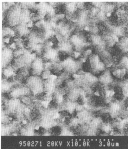
Figure 2. A scanning electron micrograph showing the surface morphology of the PbTiO 3 films on Si(001).
