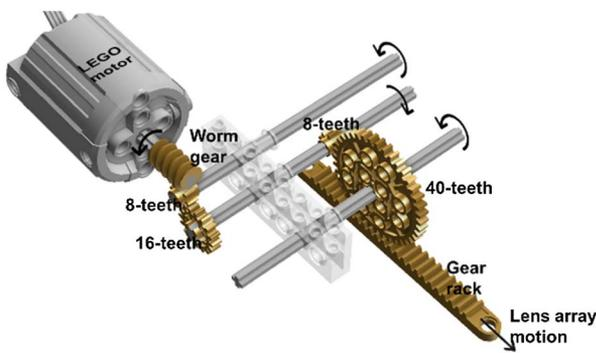
**Fig. 3.** LEGO motor and gear schematic.
