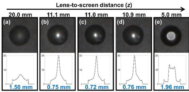
**Fig. 6.** Projected beam profile of a single lens at different  $z$  distances, showing raw image,  $x$ -axis intensity profile, and calculated FWHM (blue font). The focal length of this particular lens was 11.0 mm.
