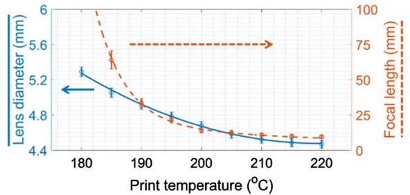
**Fig. 8.** Diameter and focal length of lenses printed with 25  $\mu\text{L}$  ( $30\times$ ) at various temperatures.
