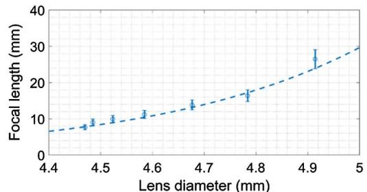
**Fig. 9.** Lens focal length versus diameter for 25  $\mu\text{L}$  ( $30\times$ ) lenses. A fit was found where  $f_{\text{Lens}} = 10^{-4} \times \exp(2.52 \times d)$ .
