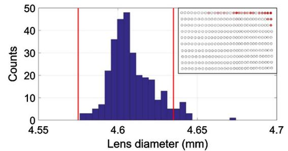
**Fig. 5.** Histogram of lens diameters: 283 of 300 lenses are within specifications of  $d = 4.61 \pm 0.03$  mm. Inset shows a color-coded image, where lenses highlighted in red did not meet specifications.
