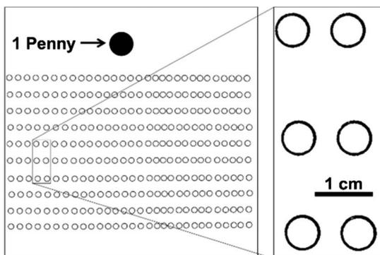
**Fig. 4.** Binarized image of as-printed 30  $\times$  lens array (30  $\times$  10 lenses).
