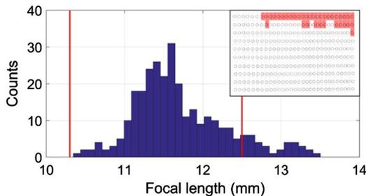
**Fig. 7.** Histogram of lens focal lengths: 265 of 300 lenses are within specifications of  $f = 11.4 \pm 1.1$  mm. Inset shows the original image overlaid with a color map to indicate out-of-specification units.
