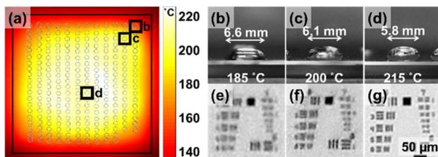
**Fig. 1.** (a) Printed lens array overlaid with temperature distribution map. (b)–(d) Three different lens diameters with corresponding printing temperatures. (e)–(g) Minimum resolvable features measured to be 35, 10, and 9  $\mu\text{m}$  corresponding to lenses in (b)–(d), respectively, using a USAF 1951 resolution test target.
