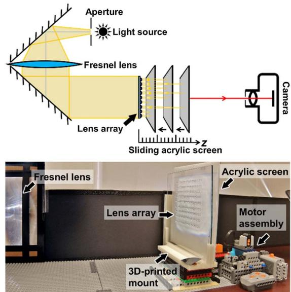
**Fig. 2.** Lens characterization system: A camera fixed behind the lens array allowed the outline of each lens to be imaged. With the addition of a motorized sliding acrylic screen, the light focused by each lens was projected onto the screen, and images of the projected beam profiles were captured by the camera. The system was assembled with LEGO bricks and 3D printed parts.
