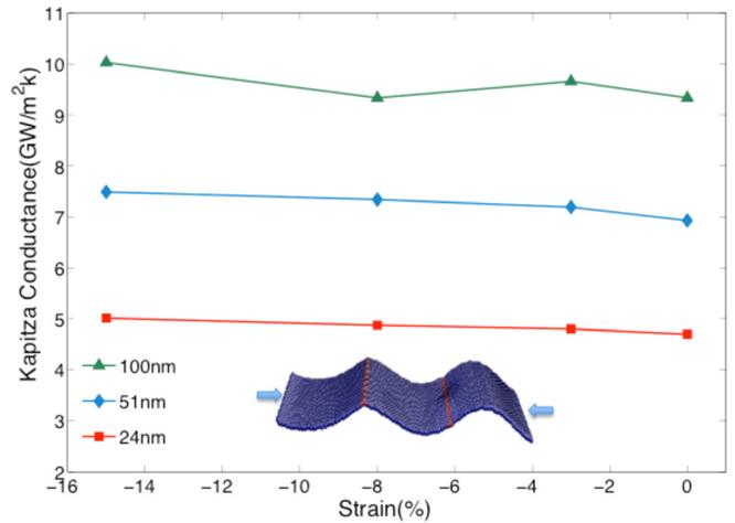
FIG. 3. Variation of the Kapitza conductance of the  $21.7^\circ$  symmetric tilt boundary in a graphene monolayer of different lengths under uniaxial compression. Inset: Deformed structure of the 24 nm specimen subjected to 3% uniaxial compressive strain.
