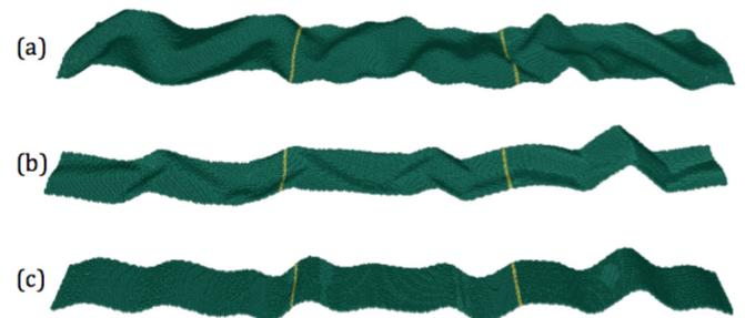
FIG. 4. Deformed structure of the 100 nm graphene specimen at 3% strain for three different cases: (a) Biaxial compression of the 10 nm wide specimen; (b) biaxial compression of the 5 nm wide specimen; and (c) uniaxial compression of the 5 nm wide specimen.
