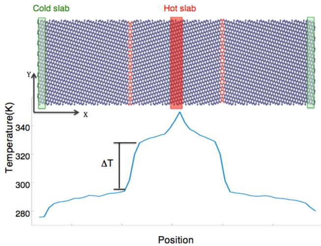
FIG. 1. Graphene monolayer in zigzag orientation (blue atoms) with two grain boundaries (red atoms). The grain boundary misorientation angle is  $21.7^\circ$ . The cold slabs on either end of the simulation cell and the hot slab in the middle are shown using green and red colors, respectively. The bottom figure shows a typical temperature profile with a distinct temperature discontinuity at the two grain boundaries.
